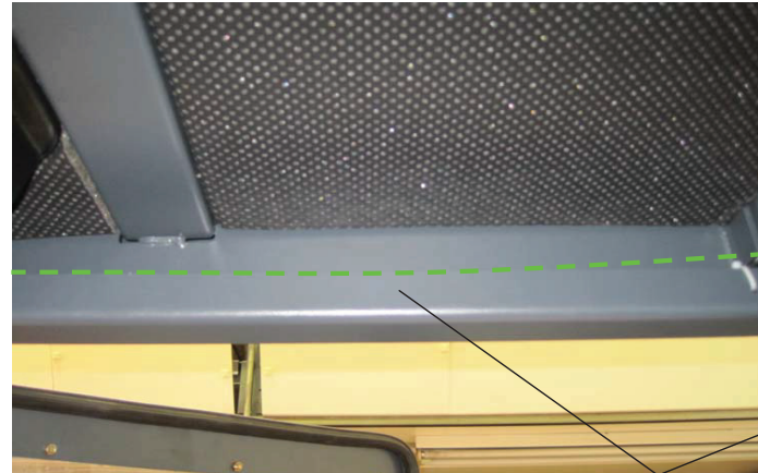
Cable harness guides W13 and W14 laid in the cab roof (right hand side)
